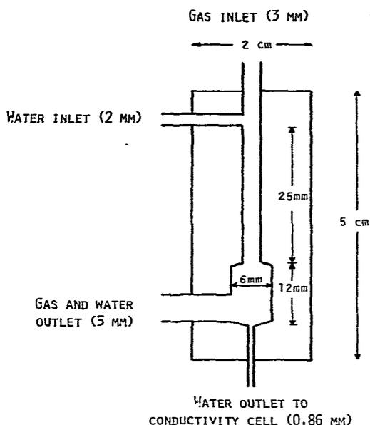
Fig. 2. Dimensions of the gas-water mixer and separator.
