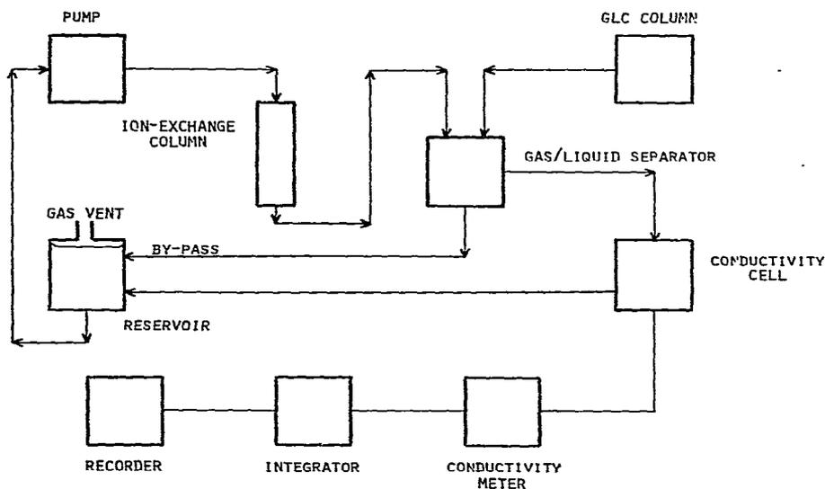
Fig. 1. Block diagram of the detector system.
